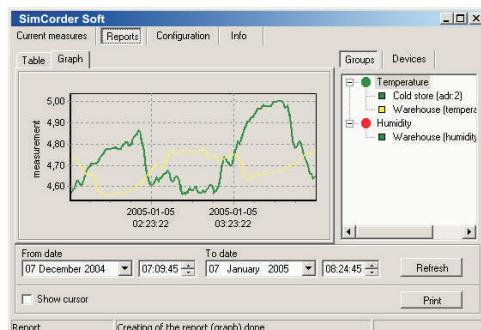
**SimCorder** software allows visualization, archiving and printing of recorded measurements. The whole measurement data is stored in special database on hard drive. Graphical presentation simplifies further analysis of the data. **SimCorder** has built in module for generation of alarms, what make managing of the processes easier for personnel. Software can operate as data server in LAN /WAN network.
