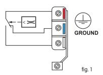
Connect to red and to white contacts of the microswitch (fig. 1). The contact red-white opens when the flow drops below the set level. When the flow is missing the contact red-blue closes and can be used as a signal or alarm contact.
