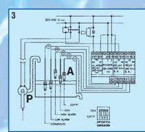
In A maintains the level between the on and off probes and activates the alarm in the liquid exceeds the "high alarm" probe.
