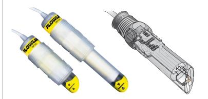
The general purpose optic leak switch provides reliable leak detection in and around secondary containment sumps, tanks and piping systems with a 1A relay output. Media examples include sulfuric acid, water and diesel. The submersible polypropylene or PFA liquid leak detection sensor is mounted through the wall or within the interstitial space.
